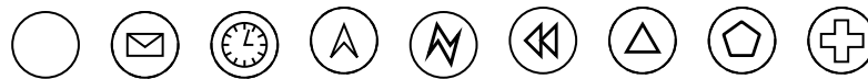
Fig. 11 Start Events – None, Message, Timer, Escalation, Error, Compensation, Signal, Multiple, Parallel Multiple
