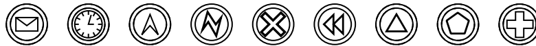
Fig. 14 Intermediate Catch Events – Message, Timer, Escalation, Error, Cancel, Compensation, Signal, Multiple, Parallel Multiple
