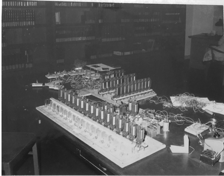
Fig. 28. Turingraum with relay shift register
