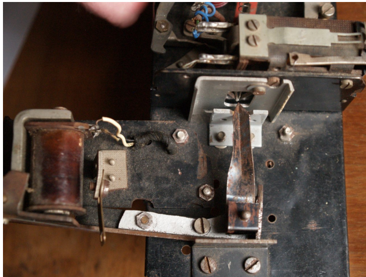
Fig. 23. Mini-Wang punch mechanism
